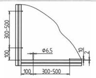
The multiblocks are installed in the clear space of the frame construction at a spacing of approx. 300 mm using cylinder-head screws M6 and rhombus nuts.
